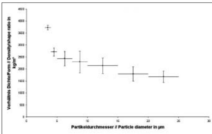
Fig. 2: Ratio of particle density to particle form for different particle size classes in a dust sample from pig fattening
