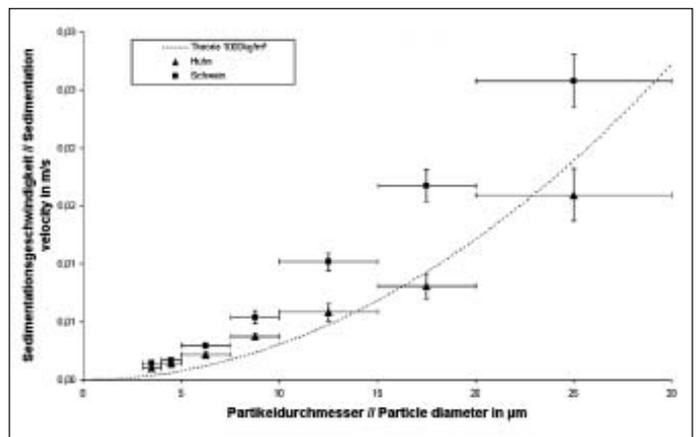
Fig. 3: Comparing measured sedimentation velocities depending on particle size classes from dust samples from pig fattening and from an aviary house for laying hens. The broken line is the sedimentation velocity of spherical particles with a density of 1000 kg/m<sup>3</sup>
