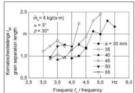
Fig. 5: Influence of frequency on the grain separation length  $l_{80}$  at different amplitudes
