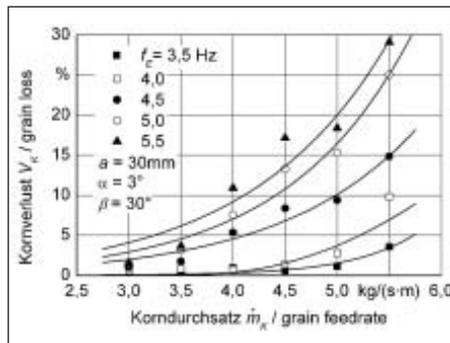
Fig. 4: Grain loss versus different frequencies
