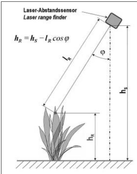
Fig. 2: Calculation of reflection height;  $h_r$  reflection height,  $h_s$  height of sensor,  $l_r$  reflection distance
