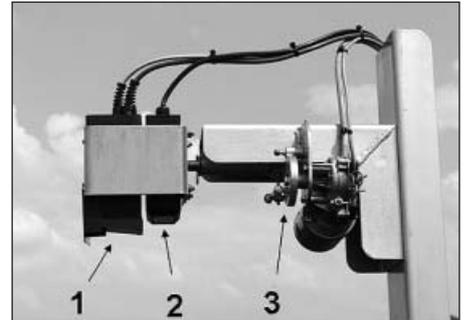
Fig. 1: Investigated laser rangefinders: 1 ACUITY-sensor, 2 LASE-sensor, 3 pivot device
