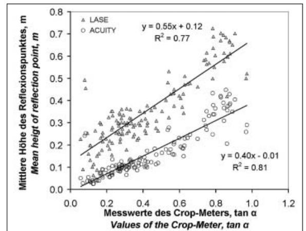
Fig. 4: Functional relationships between readings from the laser rangefinder and reference sensor
