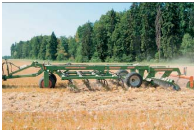
Fig. 1: Multi-beam cultivator with disc elements for shallow and for deep tillage
