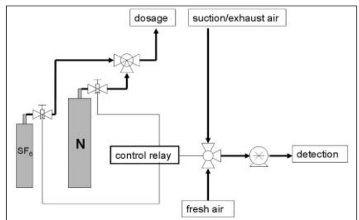
Fig. 1: Measurement setup
