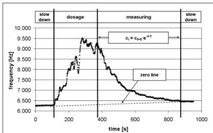
Fig. 2: Measurement cycle to calculate the ventilation rate
