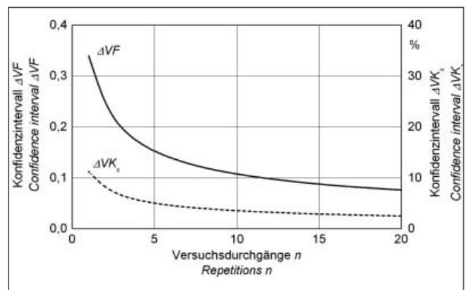
Fig. 3: Width of confidence interval variation factor VF and variation coefficient  $VK_x$  versus number of repetitions  $n$  at a confidence level of 95%
