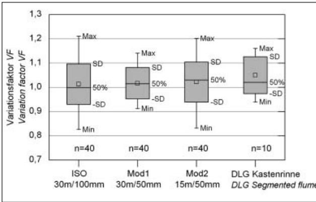
Fig. 2: Dispersion of variation factor VF at various total and segment length, calculated from 40 seed sequences and from ten empirical trials in the DLG segmented flume
