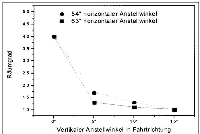
Fig. 5: Quality of residue left in seed bed after use of disc
