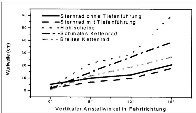
Fig. 4: Distance in which residue was displaced due to all tested tools; angle between ground surface and tool was 63°
