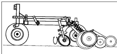
Fig. 1: Row clean tool, version 1 with device for adjusting angle of incidence
