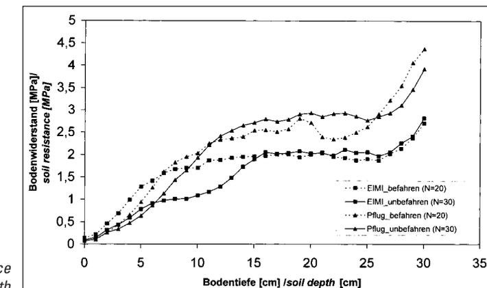
Fig. 4: Soil resistance versus soil depth
