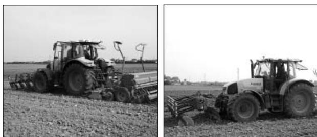
Fig. 3: Combined use of a front subsoiler with seeding combination (total weight: 9040 kg)
