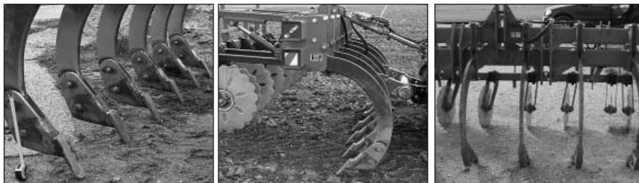
Fig. 1: Front subsoiler with rigid tines and disc coulters
