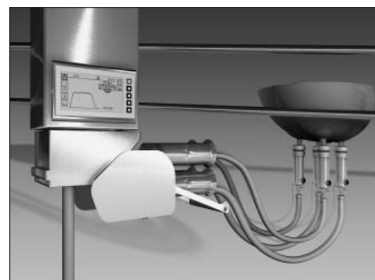
Fig. 1: The MultiLactor from Siliconform (H 24 St A25) does without a cluster clawpiece (silver medal winner)
