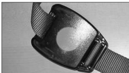
Fig. 3: The rumination sensor from Lely (H 24 St C17) for heat control was also awarded silver
