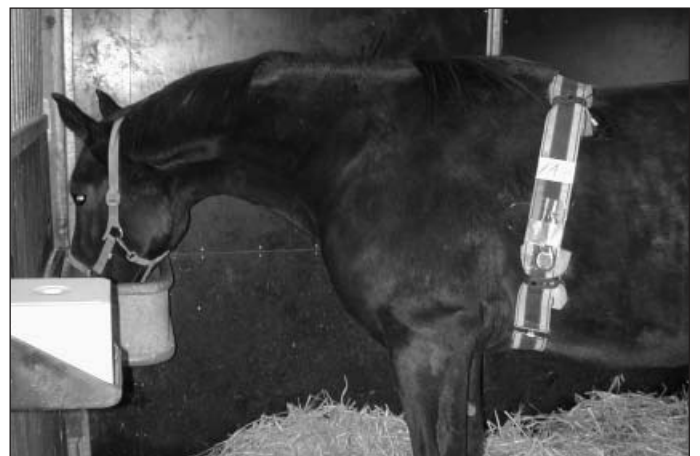
Fig. 1: Attaching of the measuring instruments (type polar Equine S810i) for recording heart frequency variability
