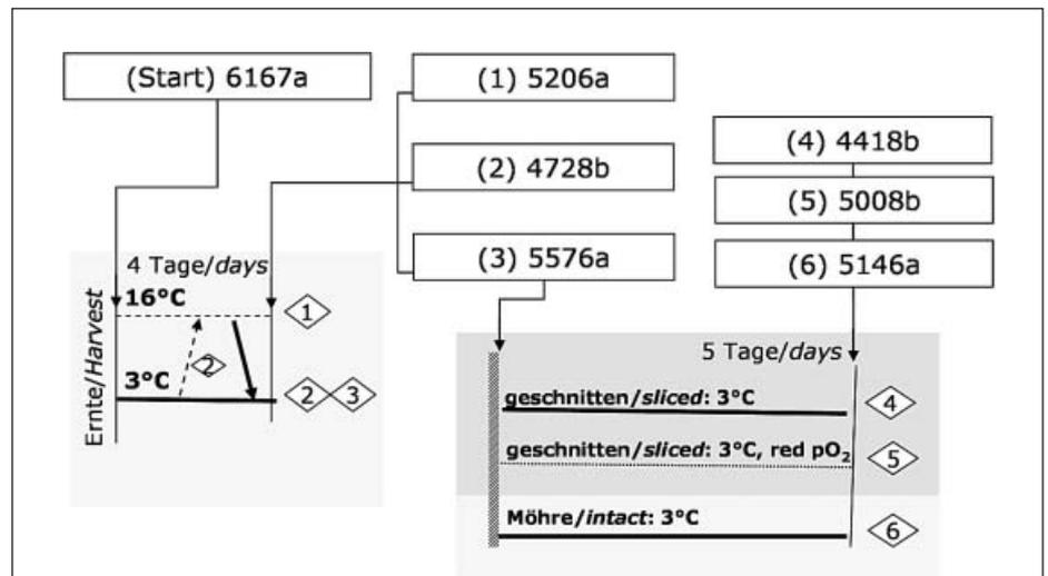
Fig. 3: Carrot  $\beta$ -carotene content [ $\mu\text{g} / 100 \text{g fw}$ ] analyzed after different postharvest conditions by means of non-destructive spectrometry. Different characters indicate significant variation at 5% level.
