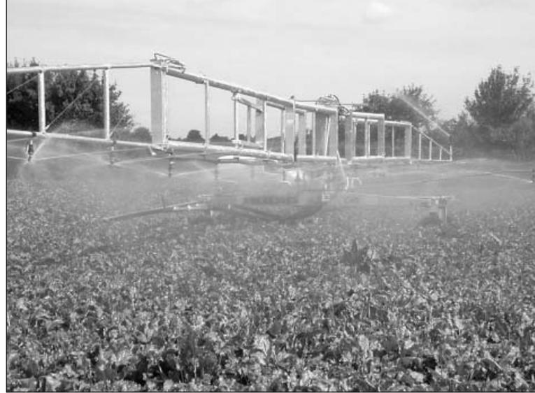
Fig. 1: Nozzle boom with 72 m working range
