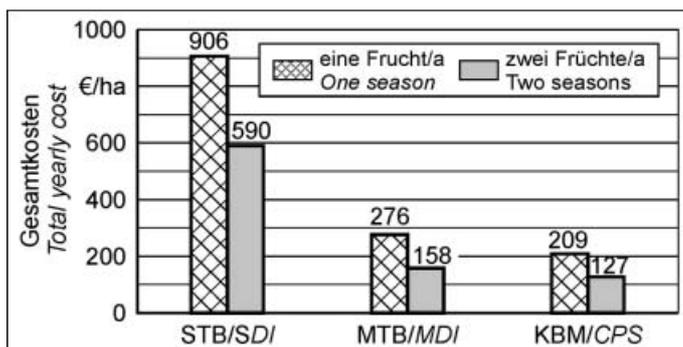
Fig. 2: Total annual costs of stationary drip irrigation (SDI), mobile drip irrigation (MDI), and a centre pivot machine (CPS). The comparison is based on an irrigated area of 50 ha.
