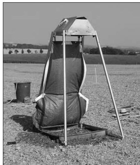
Fig 2: Used semiportable rainfall-simulator
