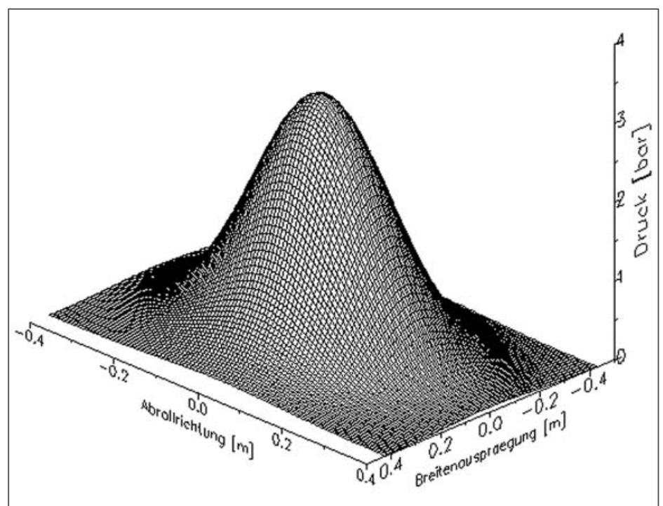
Fig. 1: Exemplary distribution of contact area pressure under a 20 cm thick sand layer
