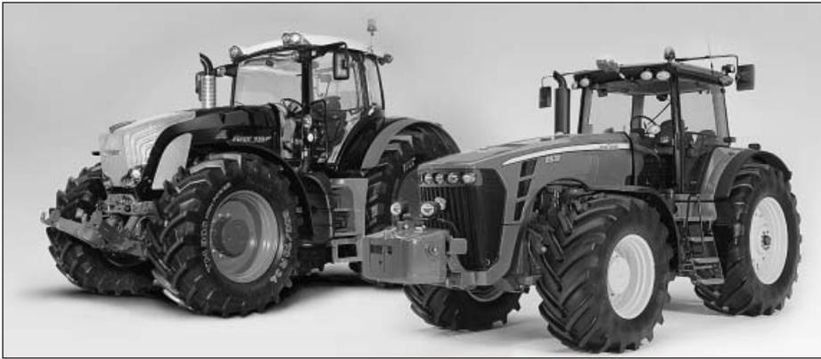
Fig. 1: Winner of the Agritechnica 2005 Gold Medals: Fendt Vario 936 (243 kW nominal ECE R24, 2006) and John Deere series 8030 (158 to 236 kW nominal ECE R24, 2006)
