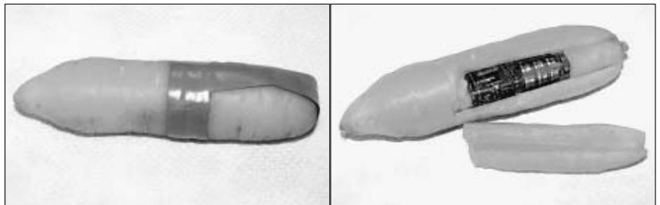
Fig. 1: Carrot with implanted data transmitter (left: carrot ready for measurement, right: carrot opened after completing measurements)
