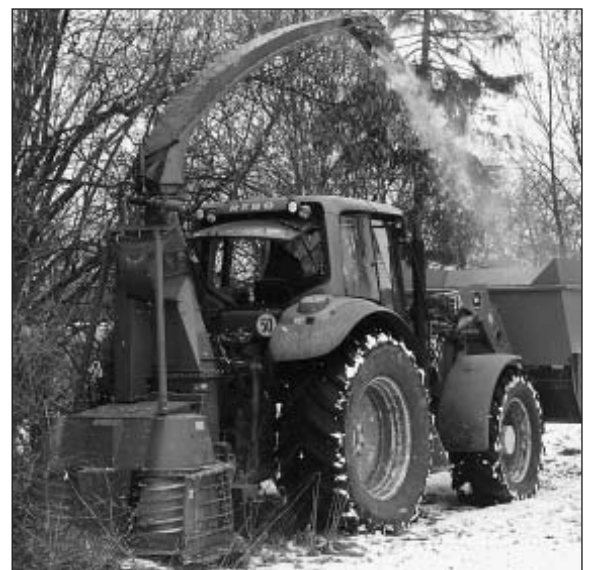
Fig. 1: First prototype of the Göttingen bush chopper „Tritucap“ with a spout
