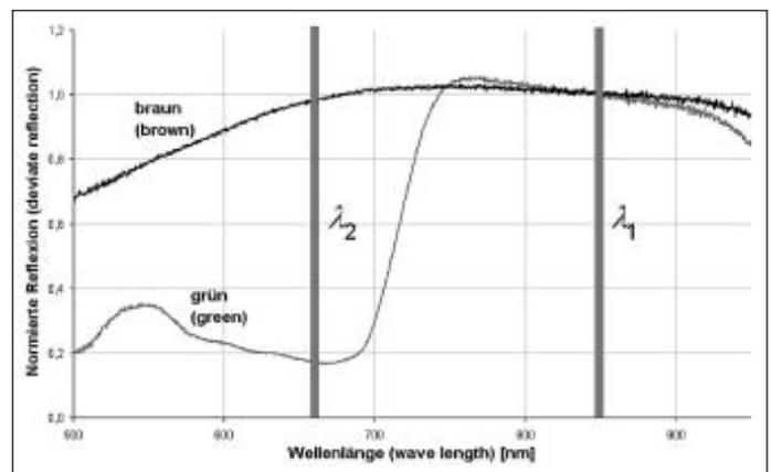
*Fig. 1: Typical spectral response of a „green“ and a „brown“ maize plant. The measurement of selective wavelengths - e.g.  $\lambda_1$  and  $\lambda_2$  - makes it possible to measure degrees of maturity.*
