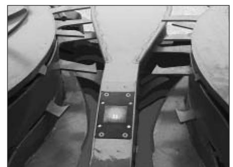
*Fig. 2: Principle of measurement for determining the degree of maturity for maize (left) and integration of the sensor system into the maize header of the BiG X forage harvester (right)*
