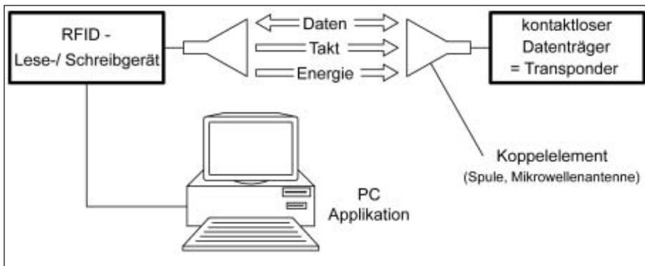
Fig. 1: Basic Modules of a RFID-System acc. to [1]
