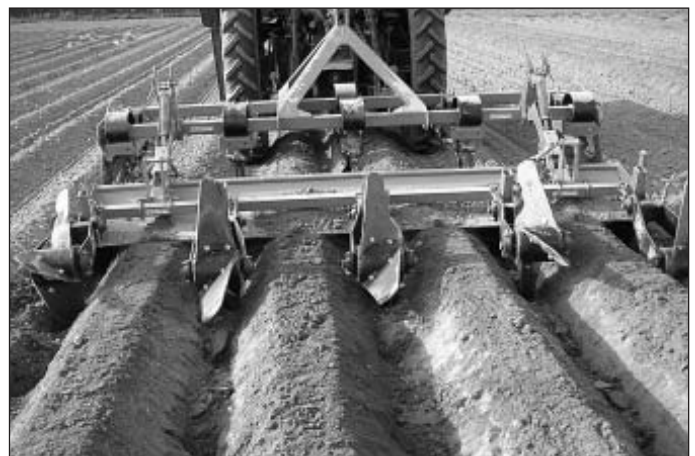
Fig. 2: Device for transversal ridging in potato furrows for better water storage
