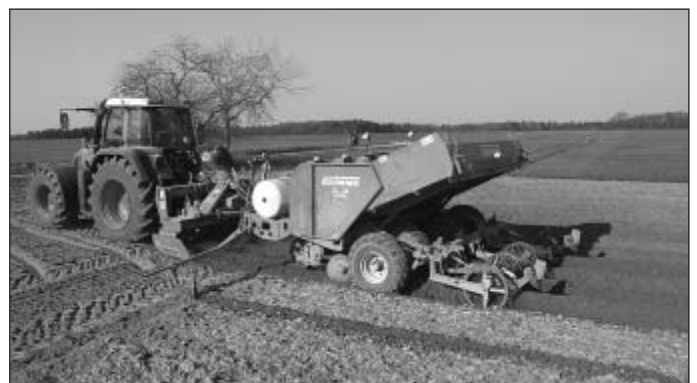
Fig. 1: In potato cultivation, plant bed preparation, planting, and ridging can be combined.
