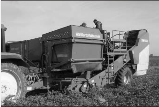
Fig. 2: Due to larger hopper capacities, one-row harvesters can increase their capacity even more.
