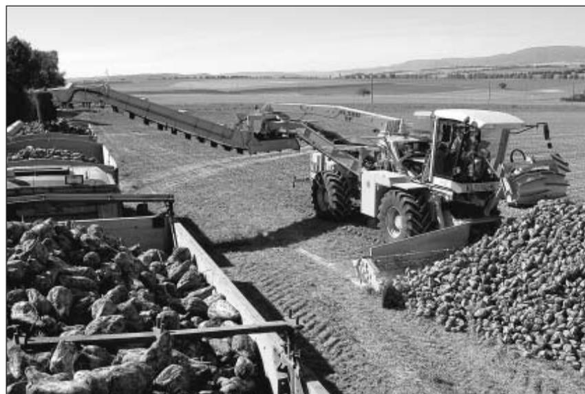
*Fig. 3: The RL 200 SF „mouse“ from Kleine loads 250 t/h at a maximum loading reach of 11.20 m (company photo Kleine)*
