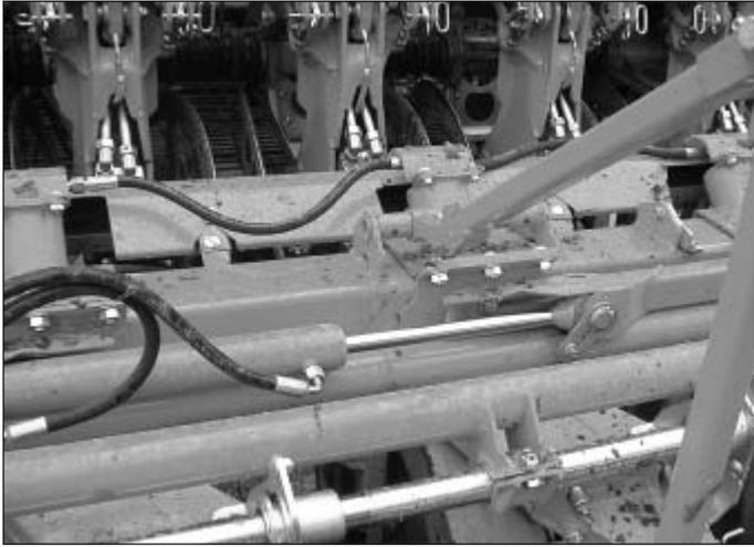
*Fig. 2: For its Maxtron 620, Grimme offers fully hydraulic row width shifting from 45 to 50 cm at the touch of a button (company photo Grimme).*
