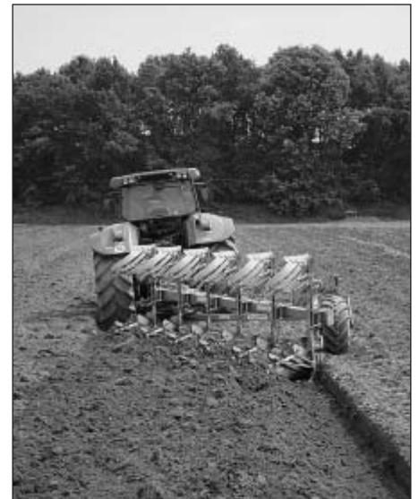
Fig. 1: In the VariTansanit, the control of the hydraulic upper link puts additional weight on the rear axle.
