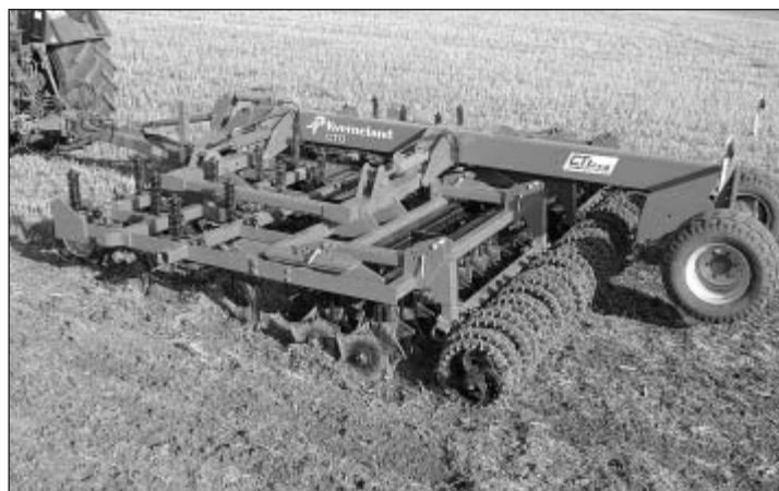
Fig. 2: Depending on the cultivator shares chosen, the CTO from Kverneland is reportedly suitable for soil cultivation from 5 to 25 cm. Two rows of rotor stars serve to crumble and reconsolidate the soil.
