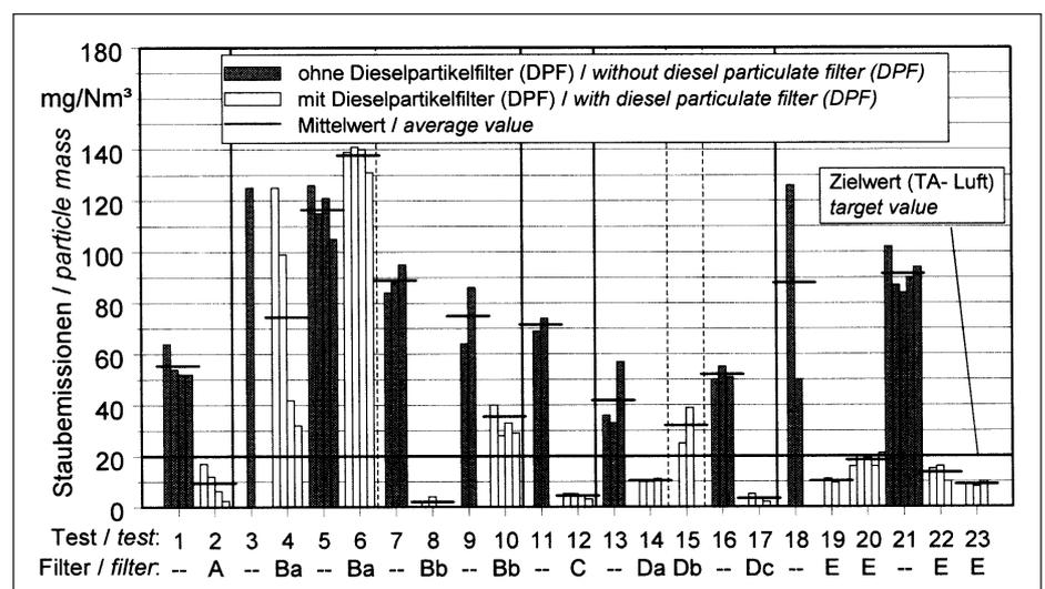
Fig. 1: Particle mass of a rapeseed oil fuelled CHP unit (8 kW<sub>el</sub>) without and with different diesel particulate filters (half-hour average values for exhaust standard conditions, 5 % O<sub>2</sub>)
