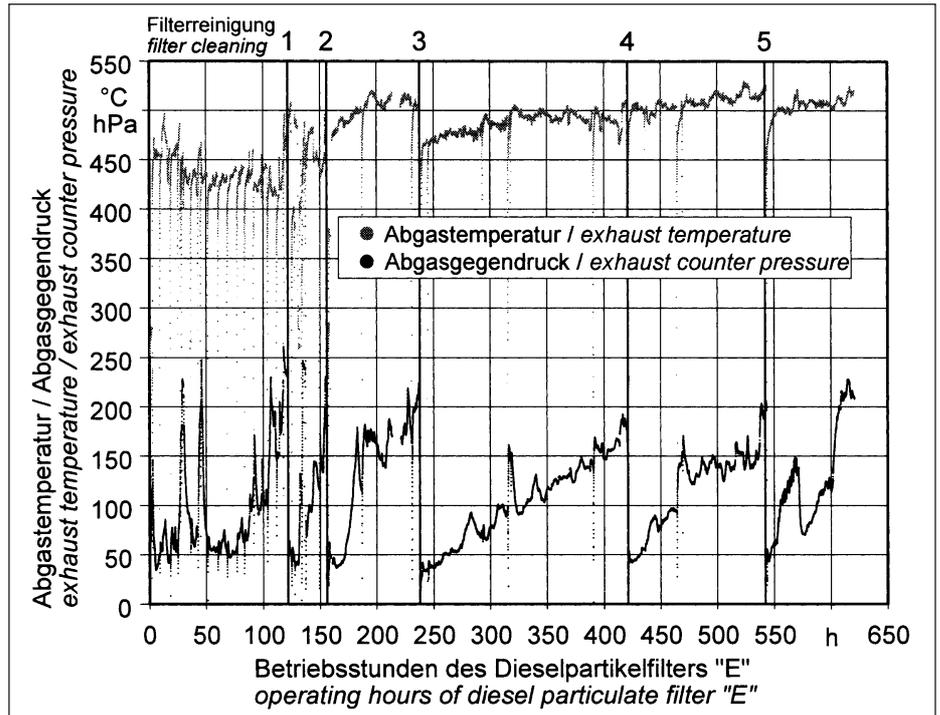
Fig. 2: Exhaust counter pressure and exhaust temperature of diesel particulate filter system „E“ over 620 operating hours with five filter cleaning interruptions
