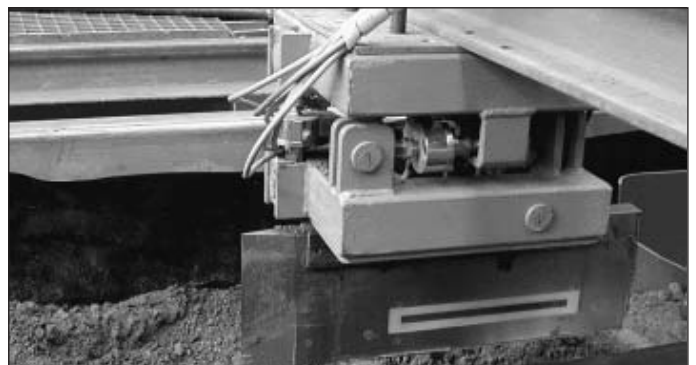
Fig. 1: Dynamic soil moisture probe within the soil bin; top: force measurement device
