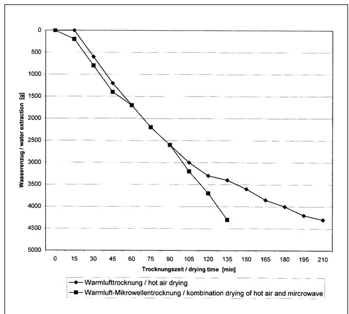
Fig. 3: Convection drying and microwave-convection drying of grain-maize, initial moisture (w.b.) 29 %, target moisture (w.b.) 14 %, inlet air temperature 125 °C, air velocity 0.40 m/s, microwave power 0.24 kW for 30 min.
