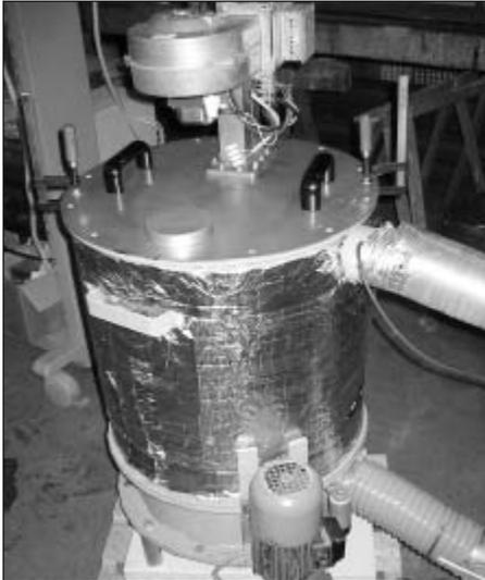
Fig. 1: Batch mixing drier
