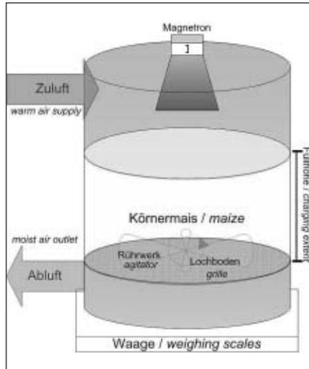
Fig. 2: Scheme of experimental drying plant
