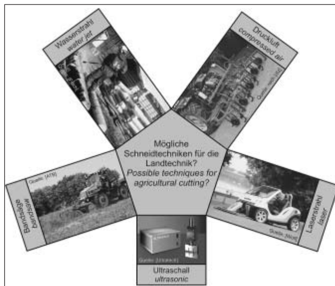
Fig. 1: Possible techniques for agricultural cutting
