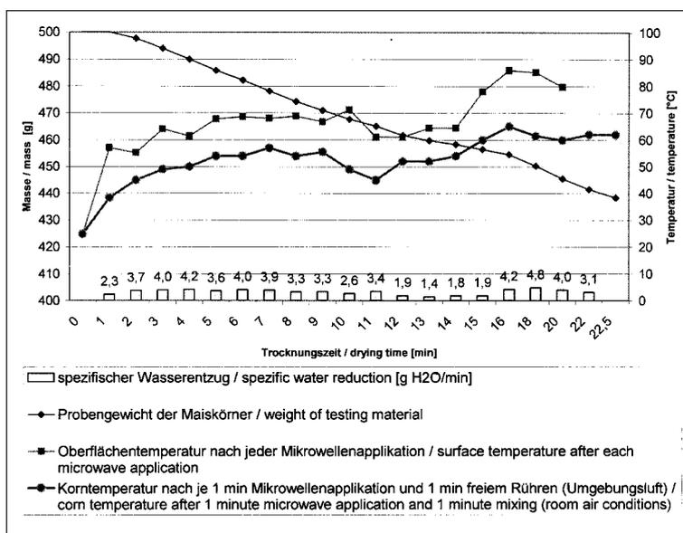
Fig. 2: Course of drying maize in microwave oven; initial moisture: 25% w.b., end moisture: 13.5% w.b.
