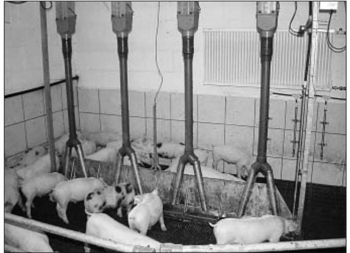
The Ferkelfeeder was developed into two different versions. One type is a double long trough with the animal-feeding place-ratio of 1 : 1, the other is a double short trough with an animal-feeding place-ratio of 4 : 1. Both were first tested and then used under practical conditions. The function of both versions is the same.
