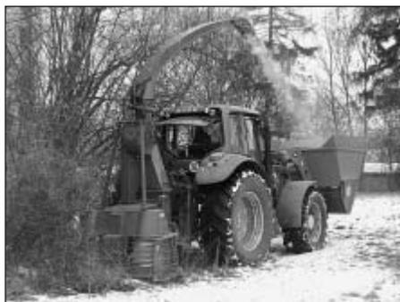
Fig. 2: First prototype of Göttingen's bush chopper „Tritucap“ with a spout
