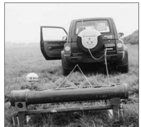
Fig. 2: Measuring instrument EM38 and transport vehicle for the measurement of soil heterogeneity
