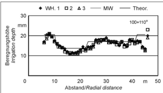
Fig. 5: Change in the irrigation depth of a centre pivot irrigator (measurement in the sector of a machine)
