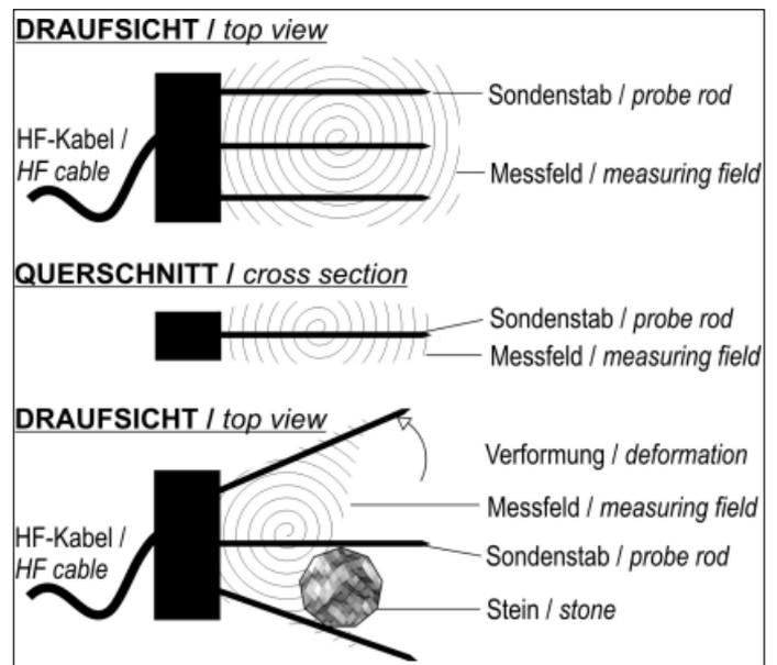
Fig. 1: Probe deformation at a 3-prong sensor
