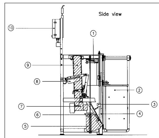
Fig. 3: Construction of the feeding station for pigs; (1) Weighing cell, (2) adjustable width, (3) antenna, (4) adjustable hole for feeding, (5) trough, (6) flap, (7) dispenser, (8) drive for flap, (9) feed store, (10) process controller with display
