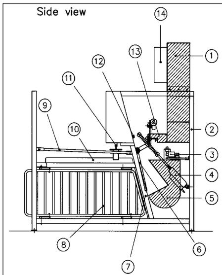
Fig. 2: Design of the feeding station for sheep; (1) feed store, (2) basic frame, (3) weighing cell, (4) drive for gate, (5) feeding trough, (6) gate, (7) front board with antenna, (8) adjustable width, (9) adjustable height, (10) swing door, (11) raster interlock, (12) light barrier, (13) dispenser, (14) process controller with display
