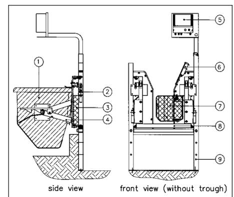
Fig. 1: Design of the feeding station for cattle; (1) Feeding trough, (2) weighing cell, (3,7) gate with interlock, (4) trough bracket, (5) process controller with display, (6) antenna, (8) weighing frame, (9) basic frame
