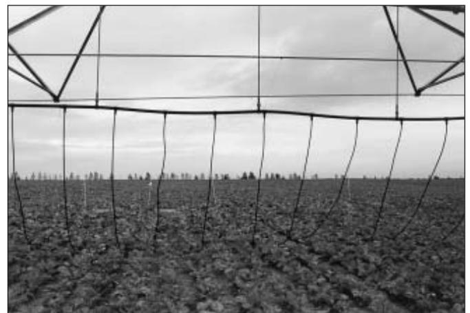
*Fig. 1: Installation of mobile drip irrigation at a center pivot irrigation machine*
