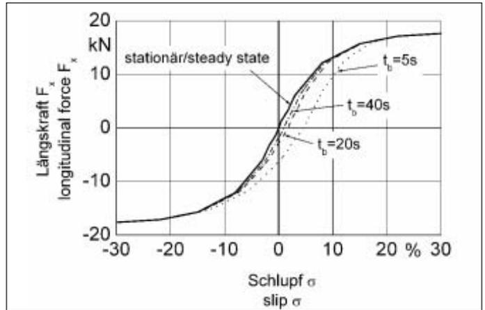
Fig. 3: Simulated longitudinal forces on a 520/70 R 34 tyre under transient slip conditions
