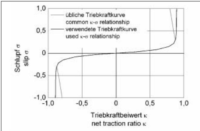
Fig. 1: Common and in the Hohenheim Tyre Model used  $\kappa$ - $\sigma$  relationship
