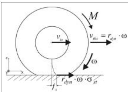
Fig. 2: Driven wheel with relevant variables
