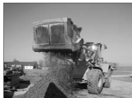
Fig. 1: Shovel processor (system Allu) at a wheel loader for picking up, transport, chopping and forming of windrow heaps
