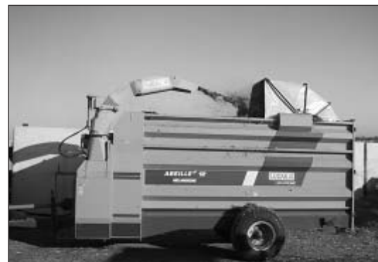
Fig. 2: Bale processor (system Lucas) at a tractor for variable chopping of horse manure and forming of windrows
