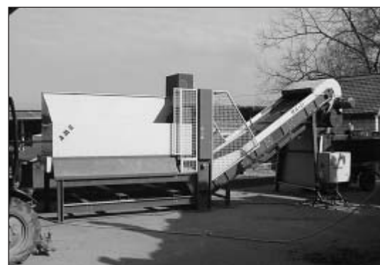
Fig. 3: Special horse manure shredder (system Wüller) powered by electric motors with dosage unit (left) and shredder (right)
