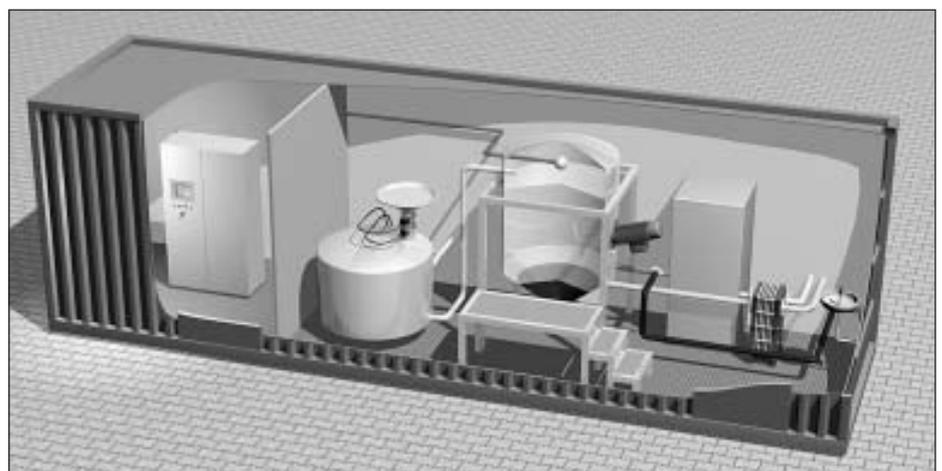
Fig. 2: All components required for decentralized biodiesel production are housed in a transcontainer.
