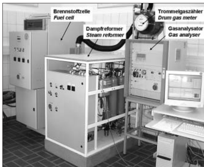
Fig. 1: Fuel cell test stand of the ATB
