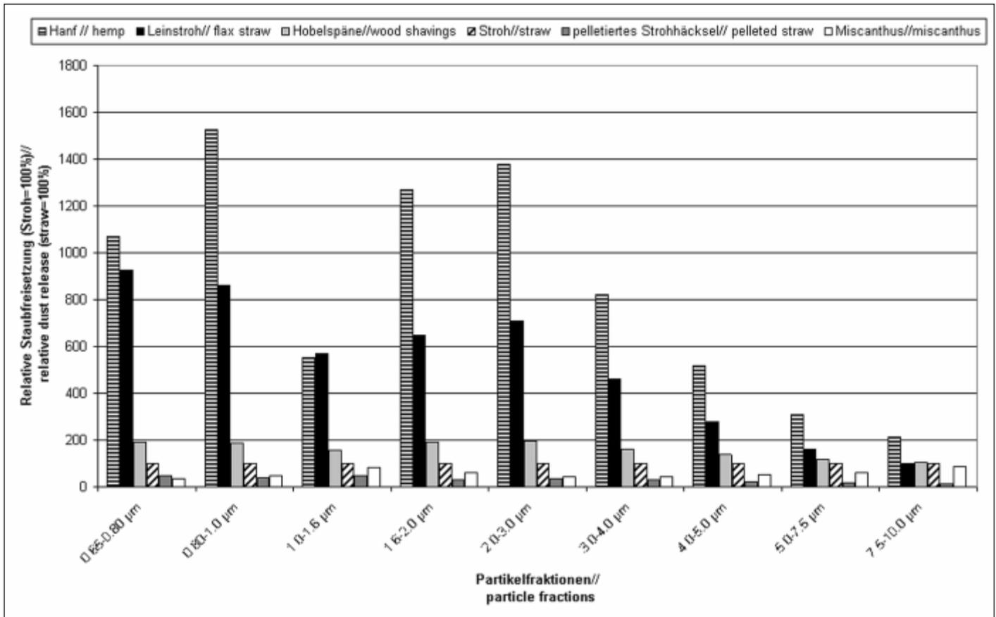
Fig. 2: Dust formation of different bedding sources in relation to straw
