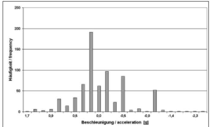
Fig. 4: Histogram of the acceleration values of the Field Scout measurements
