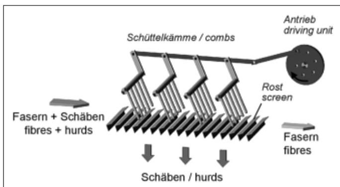
Fig. 2: Comb shaker for natural fibre cleaning
