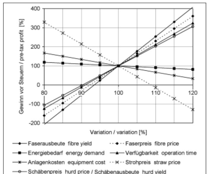
Fig. 1: Factors influencing the operation result of a fibre processing plant (100% = 65000 p.a.)
