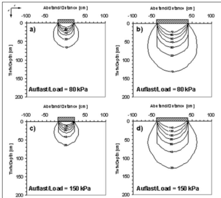
Fig. 2: Pressure bulbs (isobars in kPa) of vertical soil stresses for different wheel loads and tyre diameters. a) wheel load = 1 t,  $\varnothing = 40$  cm; b) wheel load = 4 t,  $\varnothing = 80$  cm; c) wheel load = 1,9 t,  $\varnothing = 40$  cm; d) wheel load = 7,5 t,  $\varnothing = 80$  cm
