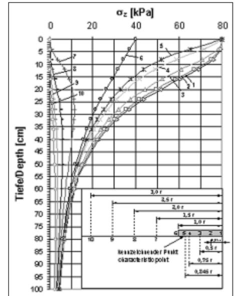
Fig. 1: Vertical soil stress function ( $\sigma_z$ ) in different distances from the load centre of a circular load area. Point 1 = load centre, point 6 = edge of tyre, point 10 = one tyre-diameter distance from the edge of the tyre
