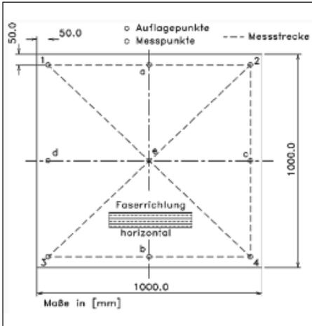
Fig. 2: Positions of measuring points on the LNS material
