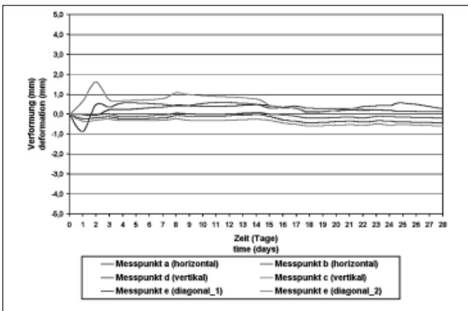
Fig. 4: Deformation of a LNS plate with cardboard-comb core
