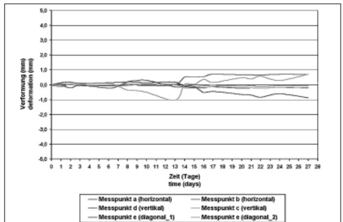
Fig. 5: Deformation of a LNS plate with triarrhena core
