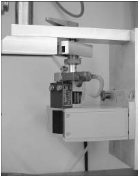
Fig. 2: Laser gauge for measuring fibre bundle diameters
