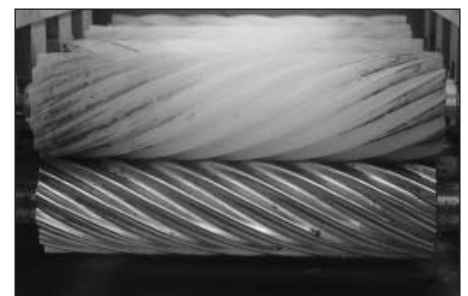
Fig. 1: Frontal view of a flax breaker
