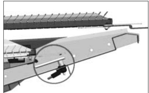
Fig. 1: Tube sensor for detection of the kernel return
