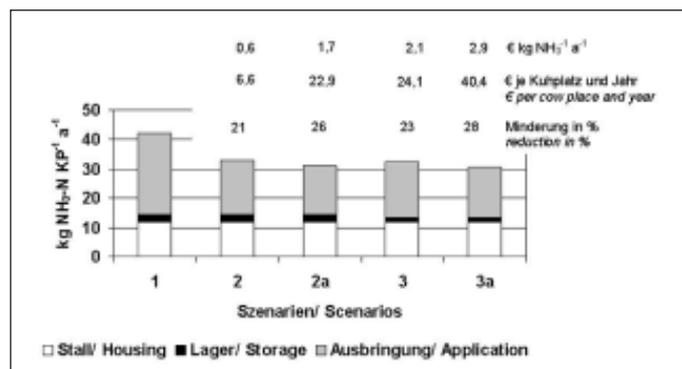
more expensive measure of covering the tank with a “tent roof” is employed (scenario 3a). With covering the slurry tank and optimised application management, ammonia emissions can be reduced by 40 % at specific cost of 0,9 € per kg of ammonia.
