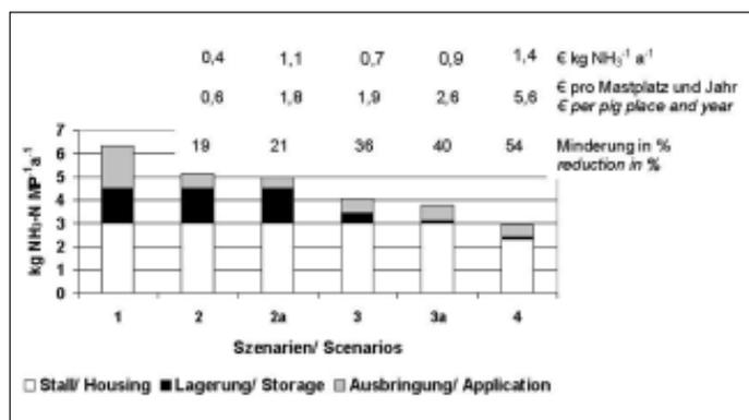
Fig. 1: Emissions, reduction in % and costs for a fattening pig housing system with 1000 places with various reduction scenarios [2]
