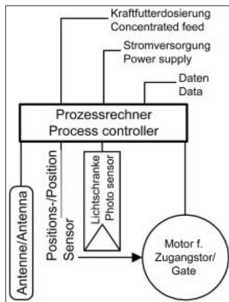
Fig. 2: Block diagramm of the feeding stations
