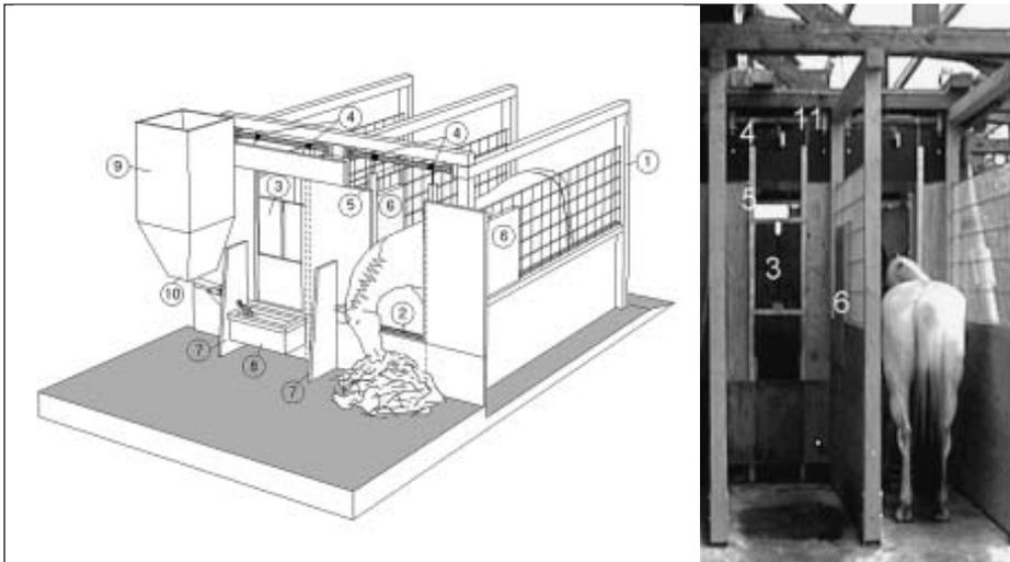
Fig. 1: Design of the feeding station (1 station partition, 2 access gate down/open, 3 access gate up/closed, 4 cable winch for access gate, 5 guide bar for access gate, 6 antenna, 7 feeding place partition, 8 feed trough, 9 concentrate feed container, 10 concentrate feed dispenser, 11 photo sensor)
