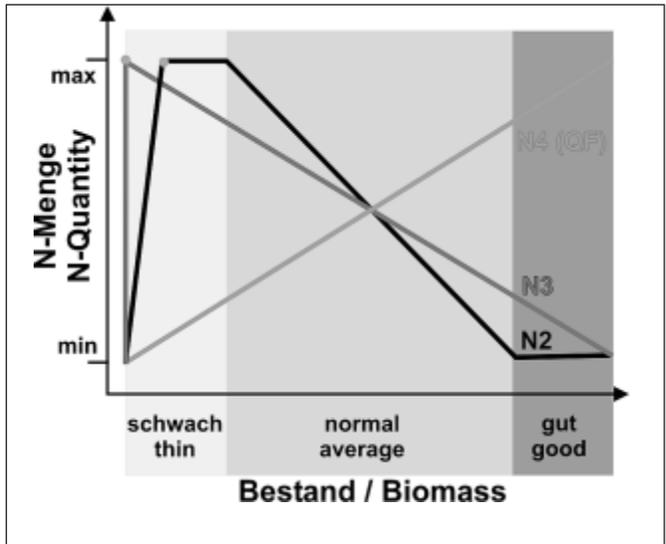
Fig. 2: Working function N-Sensor, N-quantity vs. N- status and plant growth
