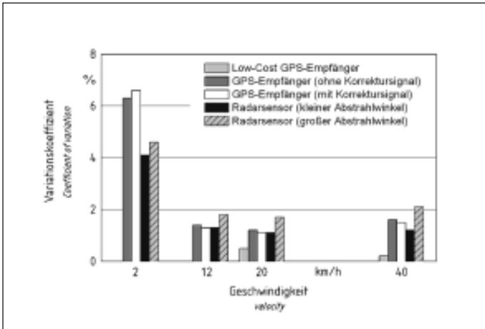
Fig. 2: Coefficient of variation of the velocity-values of two radar sensors and three GPS-receivers in relation to the velocity
